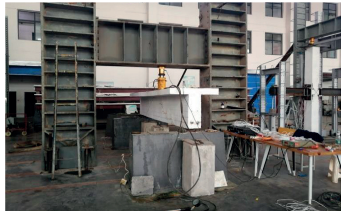
Fig. 2: Test loading device
