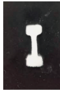
(a) Dogbone without cells Fig. 1 Sample before tensile test
